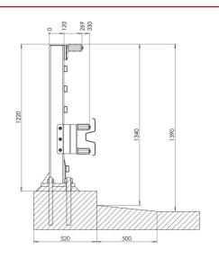
DAV H4b/W3 is primarily used onbridge structures where underlyingareas require security for extraprotection.
