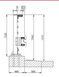
DAV H4b/W2 is primarily used on bridge constructions where underlying areas require enhanced protection.
