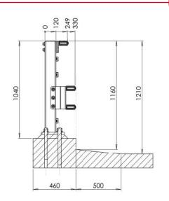
DAV H2/W2 is used on bridge constructions where normal requirements apply for a CE-marked bridge guardrail.
