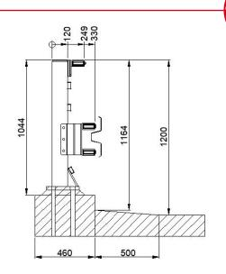
DAV H2/W1 is used on bridge constructions where normal requirements apply for a CE-marked bridge guardrail.
