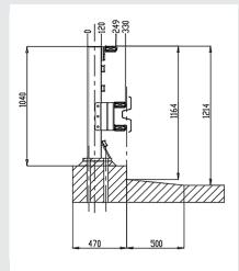
DAV H2/W1 is used on bridge constructions where regular requirements are set for a CE marked bridge guard.
