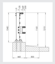
DAV H2/W3 is used on bridge constructions where regular requirements are set for a CE marked bridge guard.
